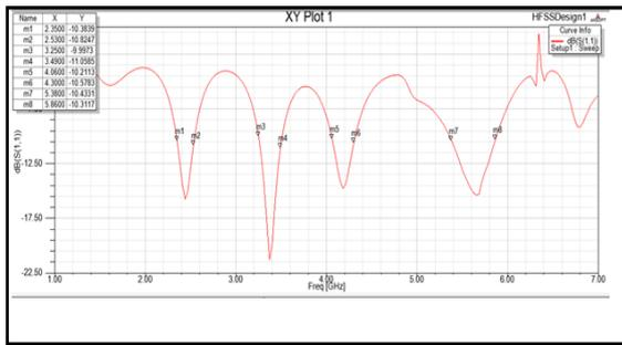
Figure 3: Simulated S-Parameter Display of Proposed Antenna
